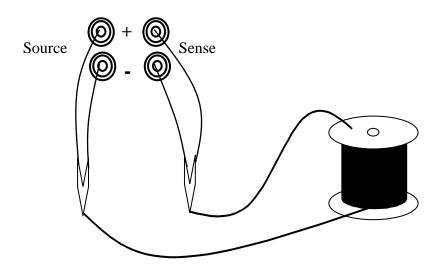
Figure 1: 4 Wire DC Resistance Measurement
