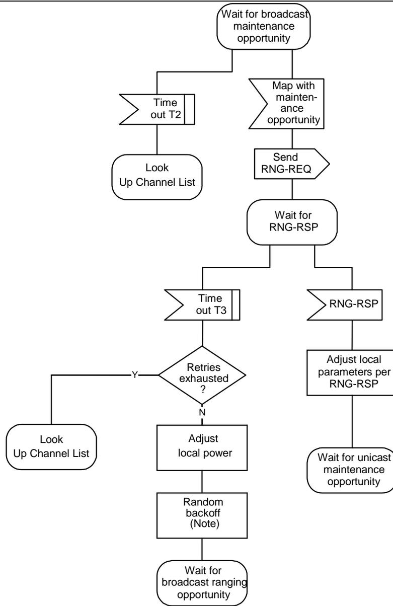
Note: Timeout T3 may occur because the RNG-REQs from multiple modems collided. To avoid these modems repeating the loop in lockstep, a random backoff is required. This is a backoff over the ranging window specified in the MAP. T3 timeouts can also occur during multi-channel operation. On a system with multiple upstream channels, the CM MUST attempt initial ranging on every suitable upstream channel before moving to the next available downstream channel.
