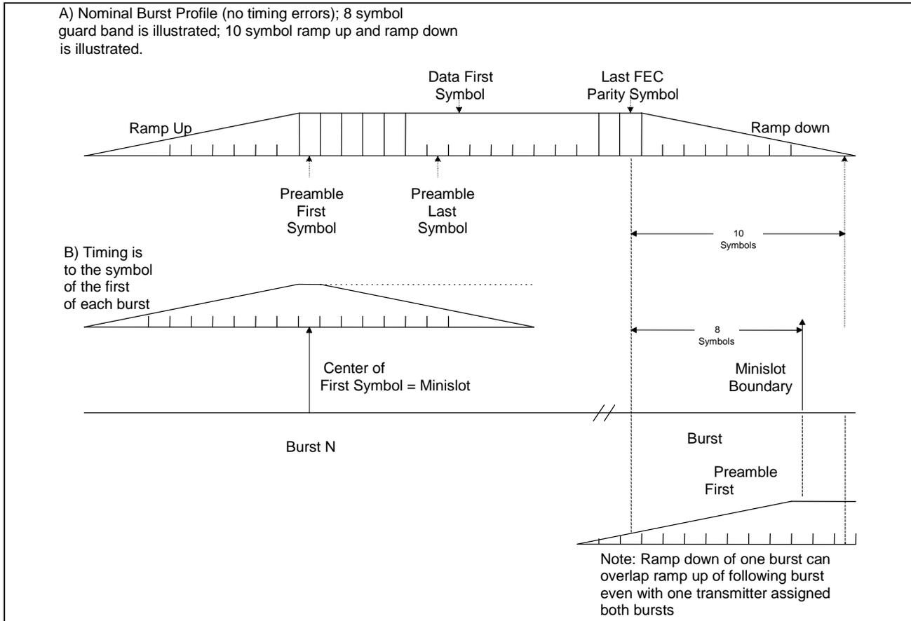
**Figure 4-6** Nominal Burst Timing
