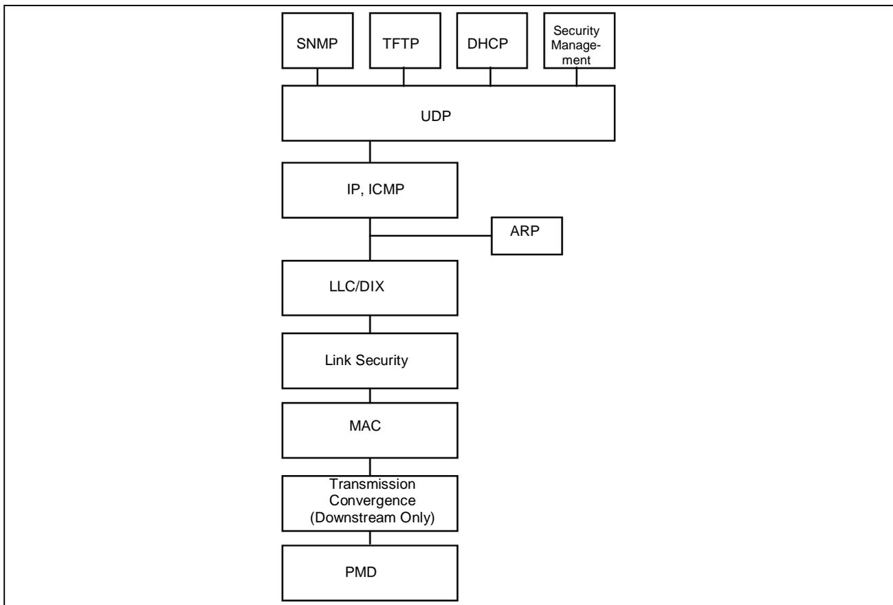
**Figure 3-1. Protocol Stack on the RF Interface**
