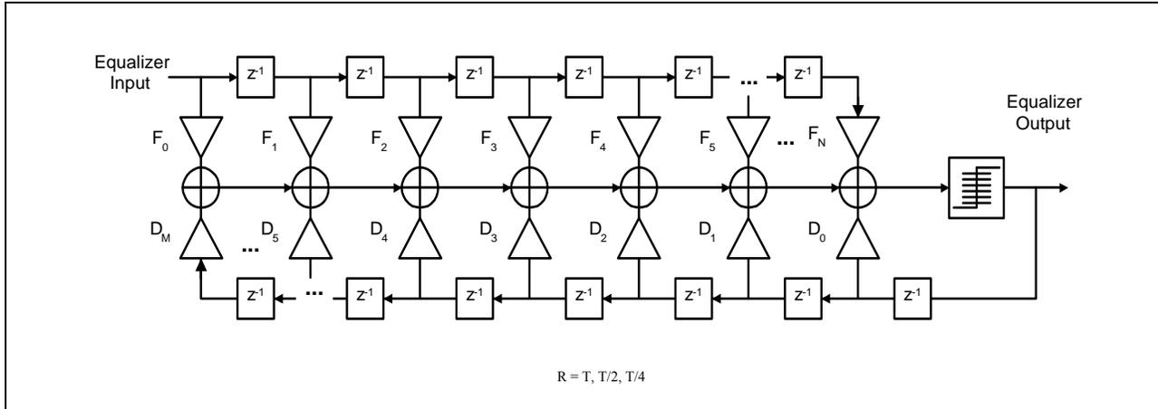
Figure 6-23. Generalized Equalizer Tap Location Definition
