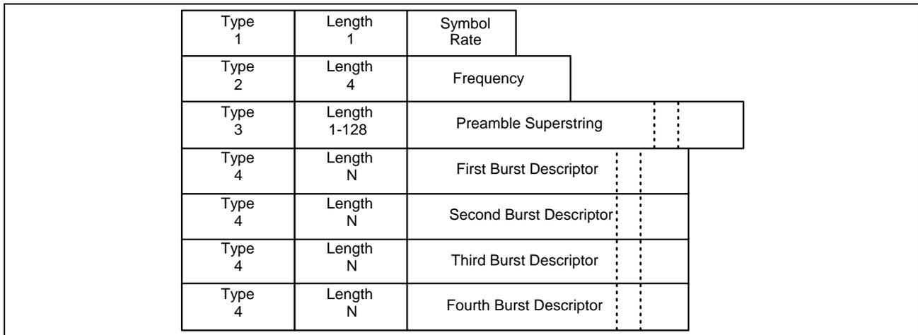
**Figure 6-17. Example of UCD Encoded TLV Data**
