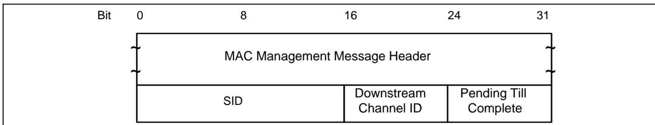
**Figure 6-20. Packet PDU Following the Timing Header**
