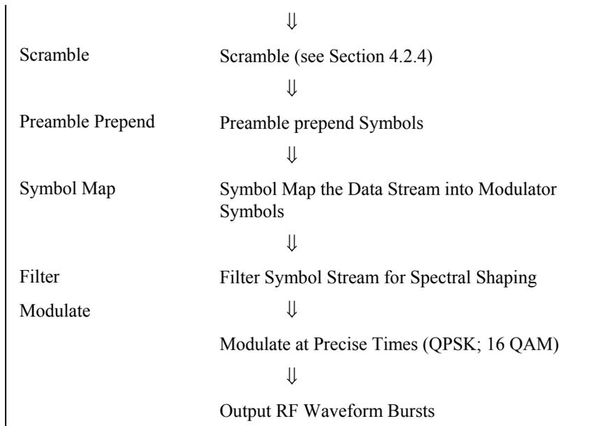
**Figure 4-10. TDMA Upstream Transmission Processing**
