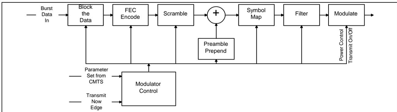
**Figure 4-9. Signal-Processing Sequence**
