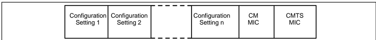
Figure C-1. Binary Configuration File Format
