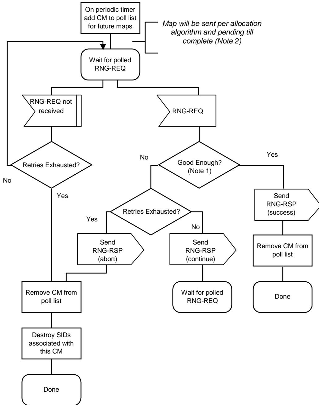
Note 1: Means Ranging Request is within the tolerance limits of the CMTS for power and transmit equalization (if supported)
