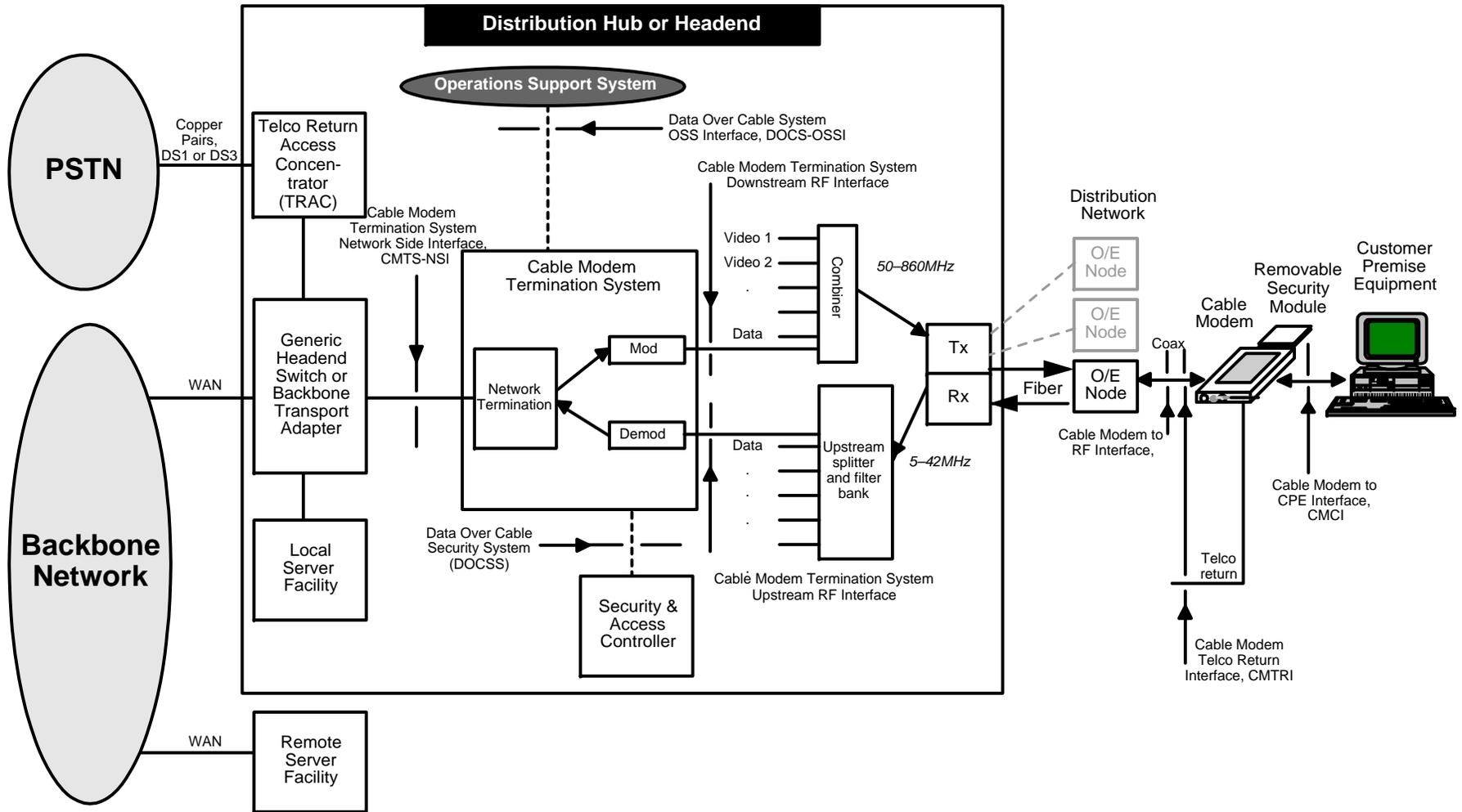
Figure 1-2. Data-Over-Cable Reference Architecture
