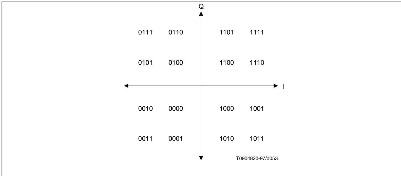
**Figure N-3. 16QAM differential-coded symbol mapping**
