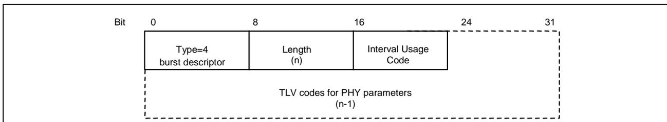
**Figure 6-16. Top-Level Encoding for a Burst Descriptor**
