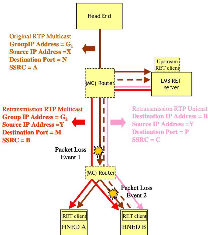
Figure 4.1: Architecture example for a RET-enabled LMB service
