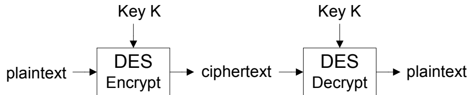
Figure B.1 FIPS 46-2 56-bit single DES.
